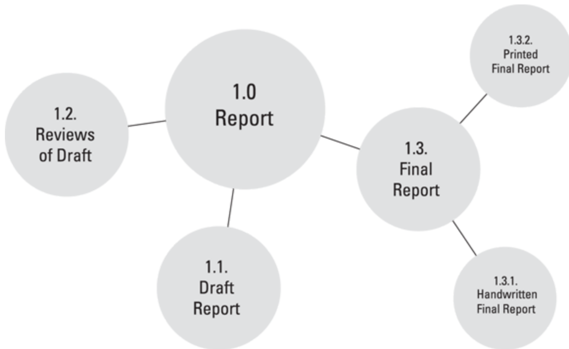
FIGURE 6-10: Drawing your WBS in the bubble-chart format.
