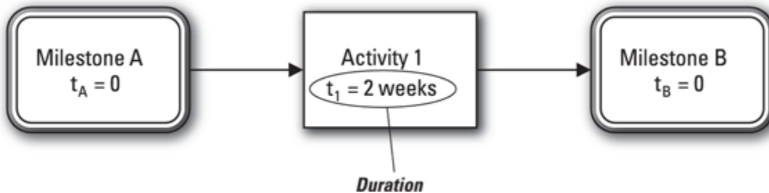
FIGURE 7-1: The three symbols in an activity-on-node network diagram.
